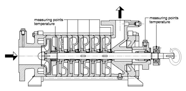
Figure 1: Points of Measurement at the SERO Test pump
