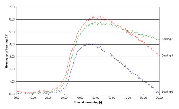
Figure 2: Heating up of bearings for operation without delivery
