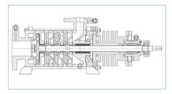
When mounting the centrifugal impellers, either one or two, in a series connection with one or more Side Channel Stages, the specific favorable characteristics of the two delivery principles complement one another.
