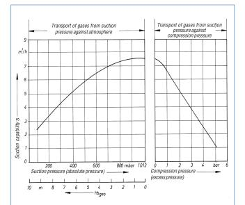
The above illustration shows a side channel pump's characteristical suction ability curve at air suction. The data depend on pump size and number of stages. During the suction period the pump works in this range until the liquid level increases due to a vacuum in the pump. For a short time a gas/liquid mixture is pumped until the pump reaches its stationary liquid flow.
