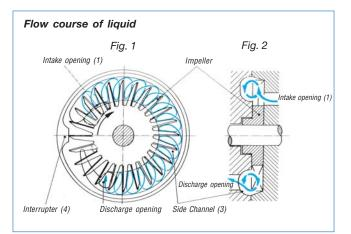
The centrifugal effect of the impeller separates air from the liquid. The liquid collects in the outer region of the impeller cells and side channel, whereas the air builds up in the inner part (5). The higher pressure in the vicinity of the discharge opening forces the air through a separate air outlet (6) into the next stage and, from there, to the delivery line.
